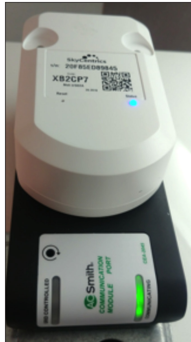
Figure 2: Photo of SkyCentrics AC Communications Module Connected to an A.O. Smith Water Heater. Photo courtesy of SkyCentrics
