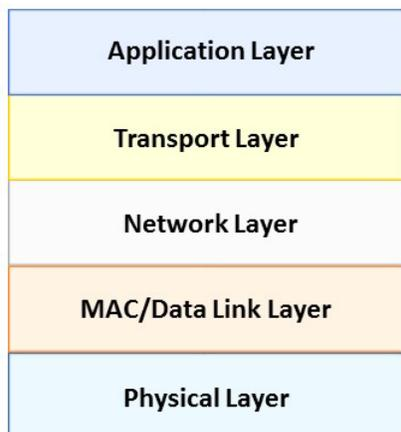
**Figure 13. Protocol stack layers for wireless sensor networks**
