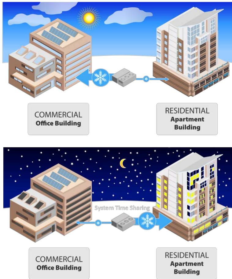
**Figure 8: Some CCs Take Advantage of Load Diversity to Minimize CAPEX**
