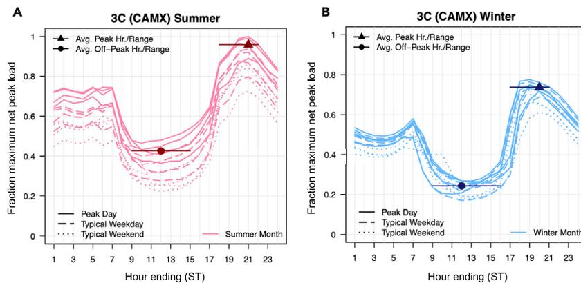
**Figure 7. Peak-normalized total system loads net variable renewable energy generation for the California (CAMX) grid region**
